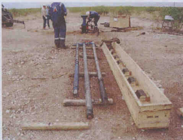
Figure 3. Motor, seal and wet connector assembly prior to being installed into lubricator.
