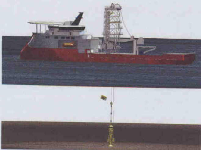
Figure 4. Rigless ESP synergy with light well intervention technology enables ESPs to be cost-effectively exploited in the subsea arena.
